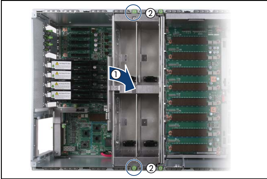
Figure 191: Inserting the fan cage
